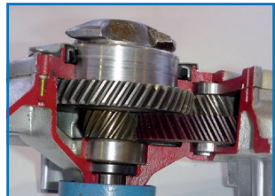
Gear transmission running in oil
