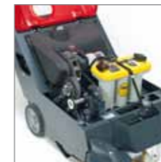
Machine interior with maintenance-free battery.
