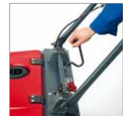
Lever for raising/lowering side brush.
