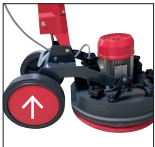
Lift the wheels off the ground to leave no running marks
