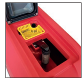
Dirty water tank with coarse dirt filter
