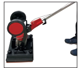
Turn the handle upside down to get max. weight on the ground
