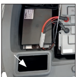
Filling opening (with bucket)
