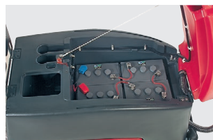
Machine open showing the batteries
