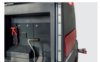
Scale for fresh water tank
