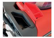
Filling hole for fresh water tank
