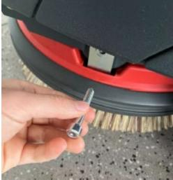
Loosen the screw on the brush head. The screw is no longer needed.
