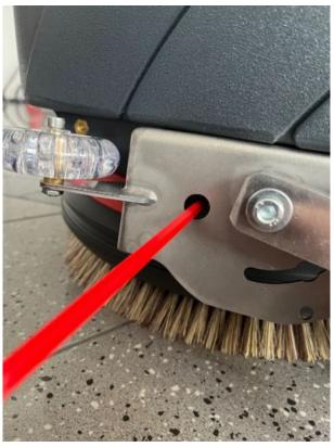
Prepare the long M8 screw with the two washers as shown and screw it tightly to pos. 1 (see page 3)
