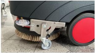
Ready-mounted transport wheel with pressure spring.
