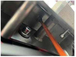
Use the M6 screw and washer to fix the transport wheel tot he fresh water tank at positions 2 + 3 (according to page 3). It may help to remove the pressure spring for this purpose (better accessibility for spanner).
